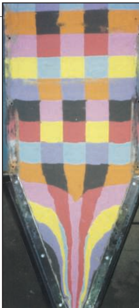
FIGURE 1. This pattern shows how the faster velocity in the center displaces material relative to the slower material at the walls
