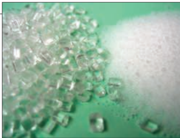
FIGURE 3. In the example described in the box on p. 44, cylindrical pellets with a nominal size of about 3 mm were being blended with nearly spherical beads with a size range from about 1 mm down to 150 microns
