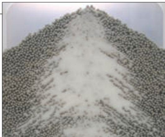
FIGURE 2. Sifting segregation occurs when a mixture containing a range of particle sizes is allowed to form a pile. Smaller particles sift between larger particles as each layer of material slides along the pile surface
