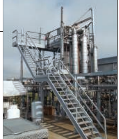
FIGURE 4. SynFuels International uses methane in pyrolysis reactors to generate acetylene, which is then hydrogenated to ethylene
